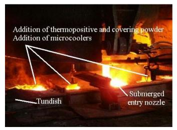
Figure 2 Places for addition thermoisolating and covering powders and of microccoolers in tundish
