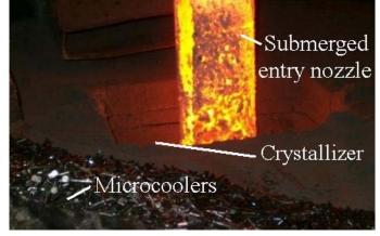
Figure 3 Places for addition of microccoolers in crystallizer
