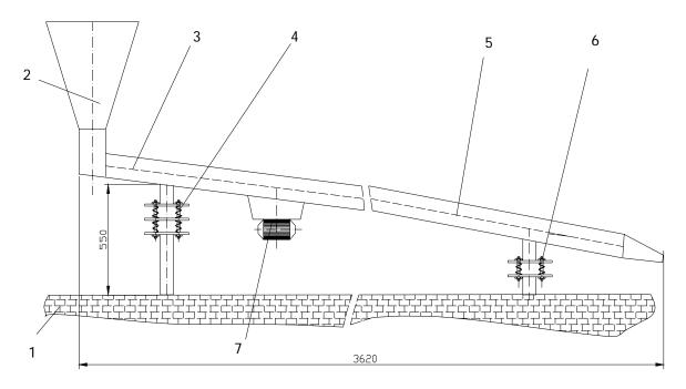
Figure 5 Experimental installation for addition of microcoolers in the tundish and crystallizer of the continuous cast installation 1- foundation, 2- bunker, 3- trough, 4, 6 - system of vibrato with spring, 5 - walls the troughs, 7 - devices of vibrato
